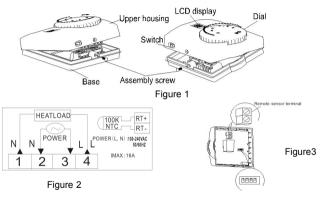
Remove assembly screws from the base of thermostat. Gently pull the upper housing straight off the base. Forcing or prying on the thermostat will cause damage to the unit. See figure 1.
